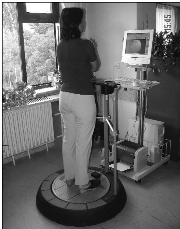
Figure 1. The subject stands on the platform during balance measurement on Kinesthetic ability trainer
